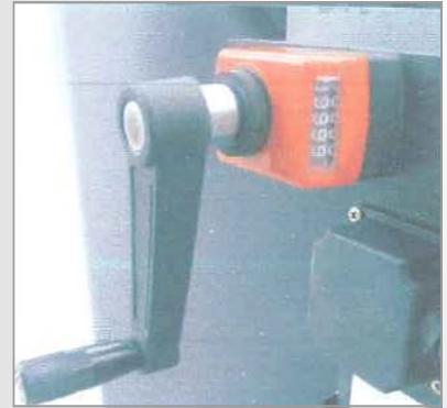
◆ Readout for boring head adjustment
